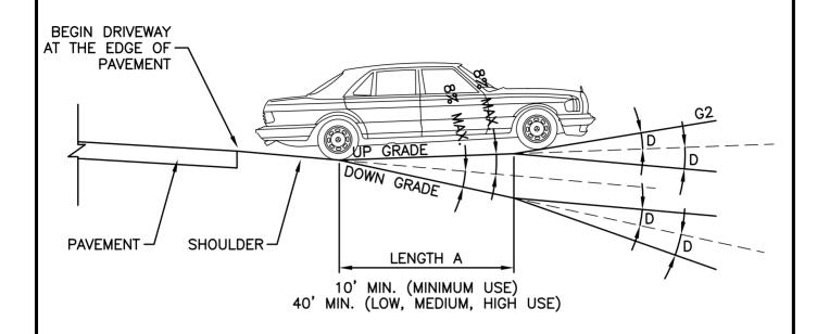
\* THE SHOULDER SLOPE USUALLY VARIES FROM 1/2" /FT. (4%) TO 3/4" /FT. (6%). HOWEVER, THE SHOULDER SLOPE SHOULD BE MAINTAINED WHEN CONSTRUCTING THE DRIVEWAY.
