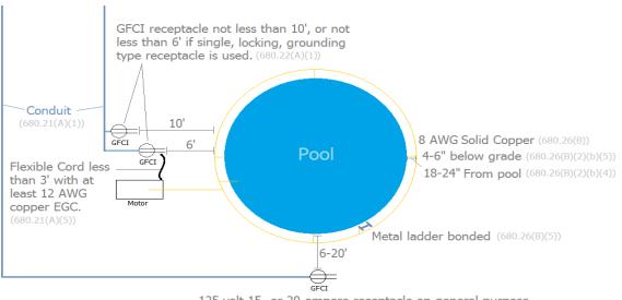
125 volt 15- or 20-ampere receptacle on general purpose branch circuit. more than 6', and less than 20' from inside wall of pool. Must be GFCI protected.  $(680.22({\rm A})(3))$
